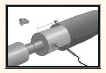
Clean exposed steel and protective sleeve and pre-heat the exposed steel and protective sleeve.
