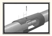
Fix the protective sleeve over casing pipe. Hole on the protective sleeve should be placed upwards.
