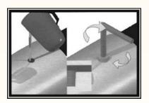
The PUR foam used to insulate seams is a Polyurethane substance made from two chemicals that are supplied in liquid form in jars or bags. The amount used varies according to the size of the seam. These amounts are given in the table Page 3.
