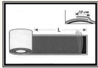
Wrap the shrink sleeve around the casing pipe, ensuring the appropriate overlap. (between the 10 and 2 o'clock position – 10cm)
