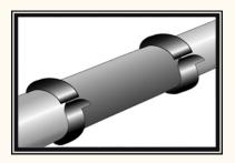
Fix the shrink sleeves. (the half of shrink sleeve should be on casing pipe, the other half should be on protective sleeve.
