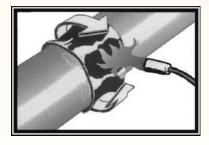
Using the appropriate torch, begin at the centre of the sleeve and heat circumferentially around the pipe.
